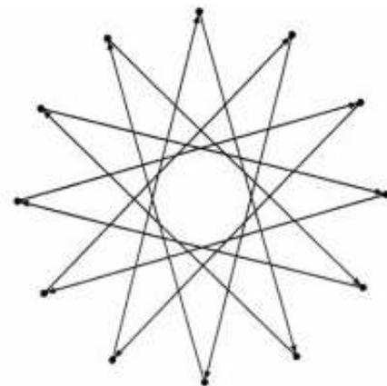
Fig. 5. 12-pointed star offers an increased path length and increased detection area.
