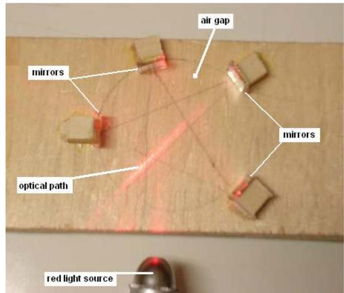
Fig. 10. Top view of a 5-pointed star optical path demonstration of concept. Phototransistor detector is not shown. The optical path length inside the air gap was measured to be 19.0 cm.
