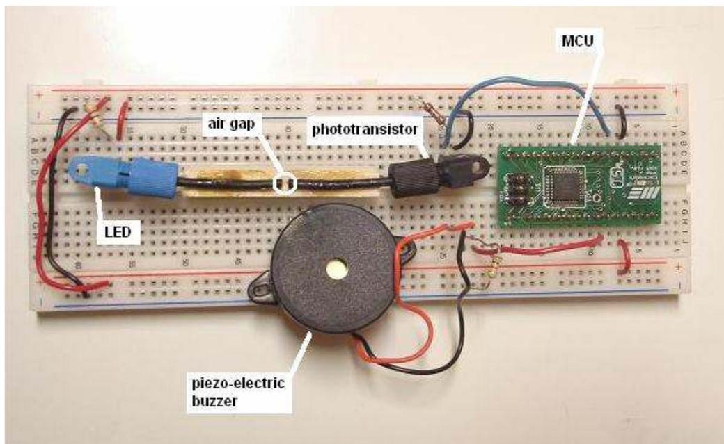
Fig. 11. Prototype of the short-distance air gap smoke detector (air gap distance = 2 mm.)
