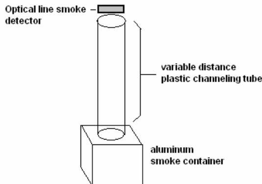
Fig. 12. General experimental setup for producing interaction between combustion particles (smoke) and the optical smoke detector. The plastic channeling tube was varied in length between 0 cm, 10 cm, and 20 cm in order to determine the operating range of the smoke detector.
