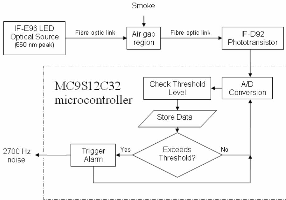
Fig. 6. Block diagram of the smoke detector with an expanded view of the MC9S12C32 programming flowchart.
