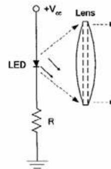
Fig. 7. Schematic diagram of the optical receiver circuit for R = 1 kΩ and using an IF-E96 plastic fiber red LED. The lens is used to focus the light onto the first incident mirror. (V<sub>cc</sub> = 5V)
