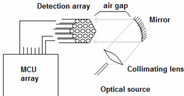
Fig. 3. A single optical transmission point is expanded and reflected to a detection array of fibers. Analysis of the optical power is performed by the MCU array.
