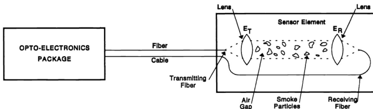
Fig. 1. Schematic of a fiber optic smoke sensor using single-light beam transmission and reception for measuring the loss of optical power due to signal degradation by smoke.
