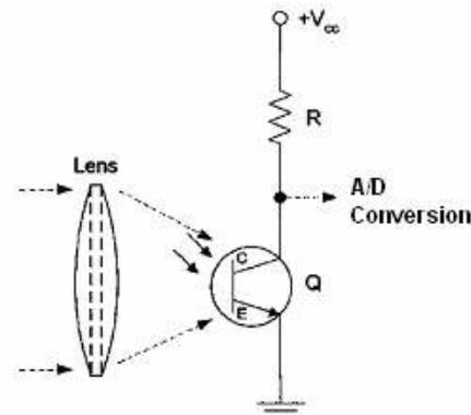
Fig. 8. Schematic diagram of the optical receiver circuit for R = 20 kΩ and Q is the IF-D92 plastic fiber optic phototransistor. The lens collects all the light from the reflected light source. (V<sub>cc</sub> = 5V)
