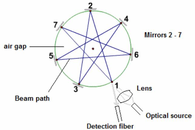
Fig. 4. A single optical transmission point is concentrated and reflected several times to increase the path length. The concentrated beam enters a detection fiber and the optical power proceeds to be analyzed by an MCU.
