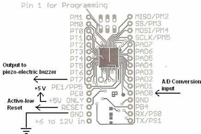
Fig. 9. MC9S12C32 16-bit microcontroller target board
