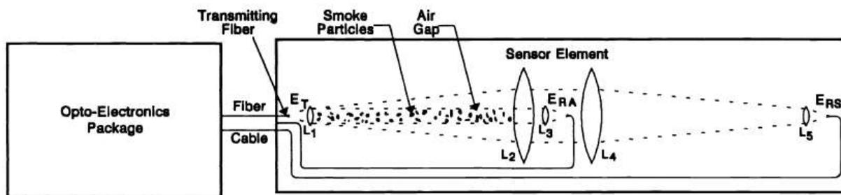
Fig. 2. Schematic of a fiber optic smoke sensor using single-light beam transmission and dual reception for measuring the optical power scattered by smoke with lens L3, and the optical absorption power with lens L5.
